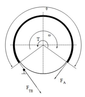
The braking torque as a function of the external brake actuation force that tightens the belt is
