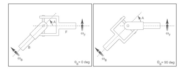
In the figure, the intersection angle is the angle between the two shafts about the pin of the base shaft. The absolute value of this angle must fall in the range  $0 \le A < Maximum intersection$  angle. The base shaft angle is the angle of the base shaft about its length axis. The base shaft angle is also the time-integral of the base shaft angular velocity,  $\omega_B$ .
