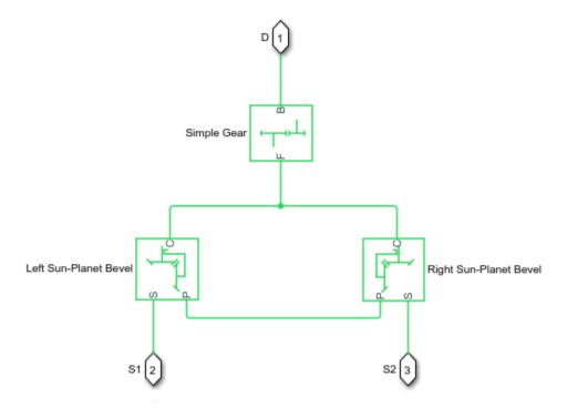
To increase the fidelity of the gear model, specify properties such as gear inertia, meshing losses, and viscous losses. By default, gear inertia and viscous losses are assumed negligible. The block enables you to specify the inertias of the gear carrier and internal planet gears only. To model the inertias of the outer gears, connect Simscape Inertia blocks to ports **D**, **S1**, and **S2**.
