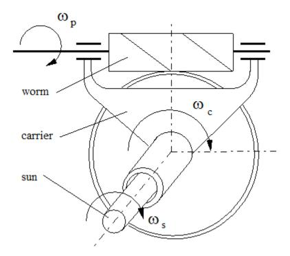
You specify a fixed gear ratio, which is determined as the ratio of the worm angular velocity to the sun gear angular velocity. You control the direction by setting the worm thread type, left-hand or right-hand. Rotation of the right-hand worm in positive direction causes the sun gear to rotate in positive direction too. The positive directions of the sun gear and the carrier are the same.
