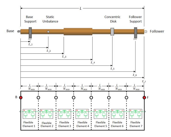
For an end-supported, axially homogenous shaft, with no static unbalances or attached concentric disks, depending on the other parameter options and values that you specify, the block might be able to solve the simulation using only  $N_{\min}$  flexible elements of equivalent lengths:
