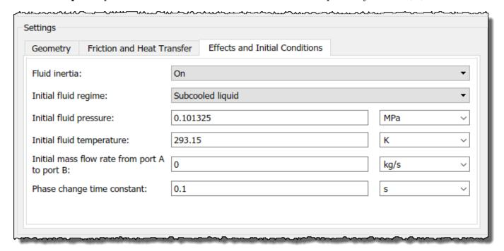
If you then change the **Initial fluid regime** parameter from Subcooled liquid to Two-phase mixture, the **Initial fluid temperature** parameter is hidden and **Initial fluid vapor quality** becomes visible. The table shows these dependencies in rows 3, 4, and 6.
