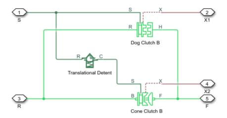
The model implements the Dog Clutch, Cone Clutch, and Translational Detent blocks. Refer to each block reference page for more information on the corresponding block function. You can use a similar approach to model customized versions of the synchronizer. One example is the Transmission (Detailed) subsystem in the model sdl vehicle manual transmission.
