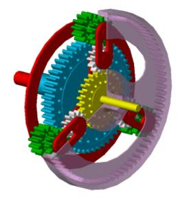
The block models the Ravigneaux gear as a structural component based on Sun-Planet, Planet-Planet, and Ring-Planet Simscape Driveline blocks. The figure shows the block diagram of this structural component.
