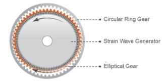
During normal operation, the base shaft drives the strain wave generator. The elliptical plug spins freely inside the elastic metal gear, propagating the strain wave about the gear rotation axis. This strain wave causes the elliptical gear teeth to engage the internal teeth of the circular ring gear progressively.
