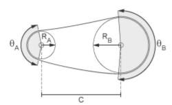
In the crossed configuration, the two wrap angles are equal and the wrap angle of the belt around each pulley is
