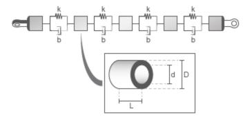
A single flexible element model exhibits an eigenfrequency that is close to the first eigenfrequency of the distributed parameter model. For more accurate analysis, select 2, 4, 8, or more flexible elements.
