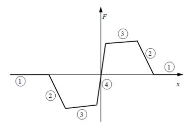
Because the ball is spherical and the notch is symmetric, the horizontal force versus displacement function is symmetric about the origin. (See "Peak Force and Notch Width" on page 1-488.)
