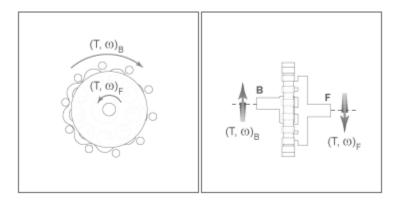
The cycloidal drive can operate in reverse mode, that is, with power flowing from the follower shaft to the base shaft. In the reverse mode, torque transfer efficiencies are typically negligible. You can adjust the efficiency by changing the value of the **Efficiency from follower shaft to base shaft** parameter.
