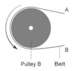
The block allows you to select the relative belt direction of motion. The two belt ends can move in equal or opposite directions. The block model assumes noncompliance in the belt and no resistance to motion due to wrapping around the pulley.
