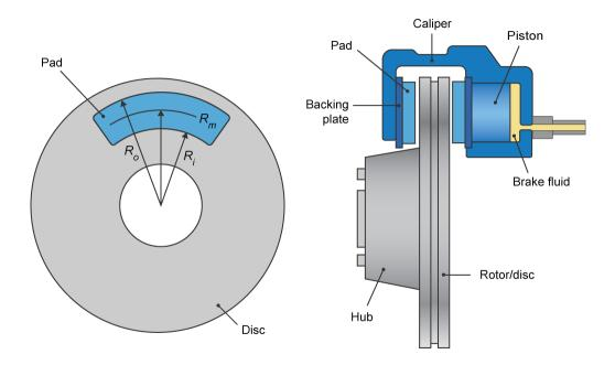
A disc brake converts brake cylinder pressure from the brake cylinder into force. The disc brake applies the force at the brake pad mean radius.
